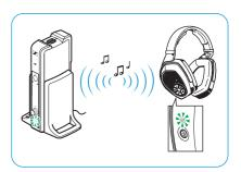
If the headphones are brought outside the transmission range or if there is no audio signal received from the transmitter for more than 5 minutes, the headphones switch off automatically.
